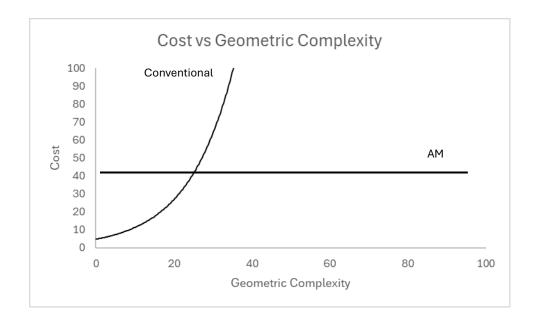
Observing the graph, one notices there is a breakeven point. This represents the point at which a part's geometric complexity contributes to its costs such that any more complexity would mean that additive manufacturing would become the more economical manufacturing method, as the conventional processes witness steep increases in cost. This increase in cost is a factor of tooling becoming more expensive and complex to produce and more processes and time needed to make the geometry.
