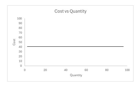
So, the cost curve for conventional manufacturing technologies is a downward sloping line which hits an eventual limit on cost per part, and the cost curve for additive manufacturing is a flat line wherein the costs of making a part are not changed by the quantity produced. The relationship between the two curves yields more information.
